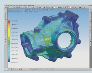
assemblies. NX Design Simulation includes the integrated NX Nastran® finite element solver, the same solver used by high-end analysts, for quick-turnaround linear structural and thermal evaluations as well as sizing and parametric shape optimization.
